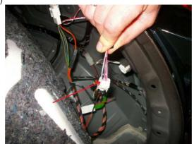
The electronic unit for the trailer lights needs supply of the fog lights in order to switch off the lights on the vehicle and thus supply the trailer lights when the plug is connected.
