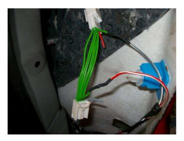
Following this modification the fog lights operate correctly on the vehicle and on the towbar plug. ATTENTION: The fog lights switch off on the vehicle on condition that the trailer is equipped with fog lights (no switch on the plug).
