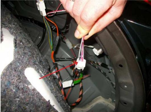
The electronic unit for the trailer lights needs supply of the fog lights in order to switch off the lights on the vehicle and thus supply the trailer lights when the plug is connected. This information is possible through 2 by-passes on the towbar harnesses (wires marked by the arrow on the photo):
